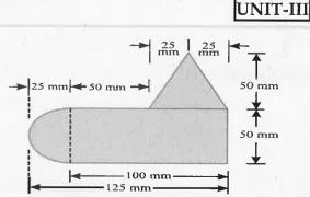
A uniform lamina shown in Fig consists of a rectangle, a circle and a triangle. Determine the centre of gravity of the lamina. All dimensions are in mm
